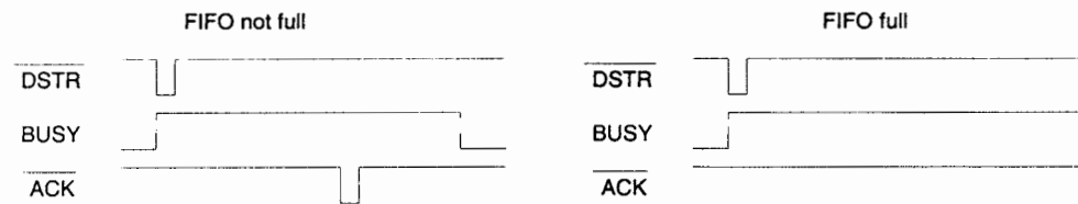
Figure 2.3. Handshake on Acknowledge, Acknowledge Before Busy
